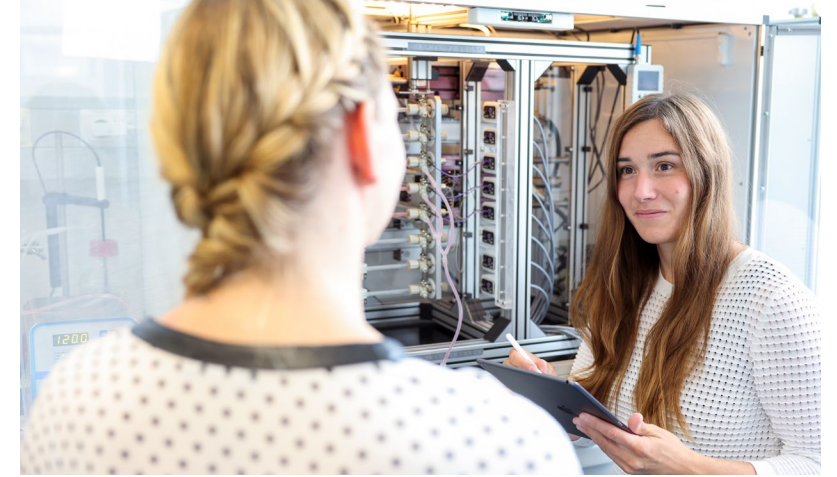
Test setup for multi-axial fatigue testing for characterization of the isolation properties of pace maker leads or peripheral stents, respectively; an internationally recognized in-house development of the IIB e.V.
