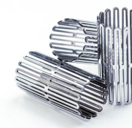
Process steps in the manufacturing of stent structures using femto-second laser cutting – from cutting the raw tube materials to mechanical post-processing and shaping through thermal treatment
