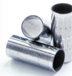
Process steps in the manufacturing of stent structures using femto-second laser cutting – from cutting the raw tube materials to mechanical post-processing and shaping through thermal treatment
