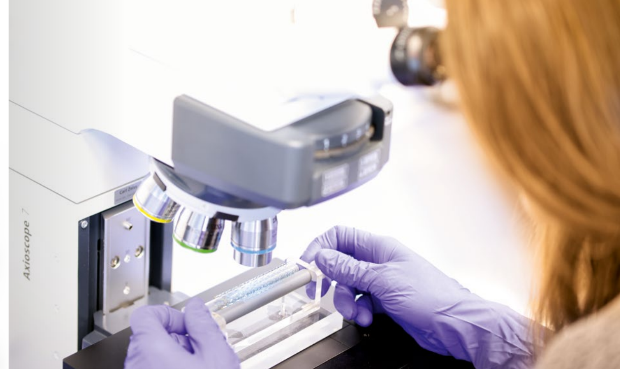
Optical microscopic analysis of stents and their coating as quality control
