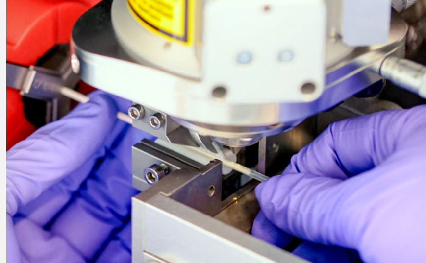
Cutting and microstructuring of polymers and metals using femto-second laser technology
